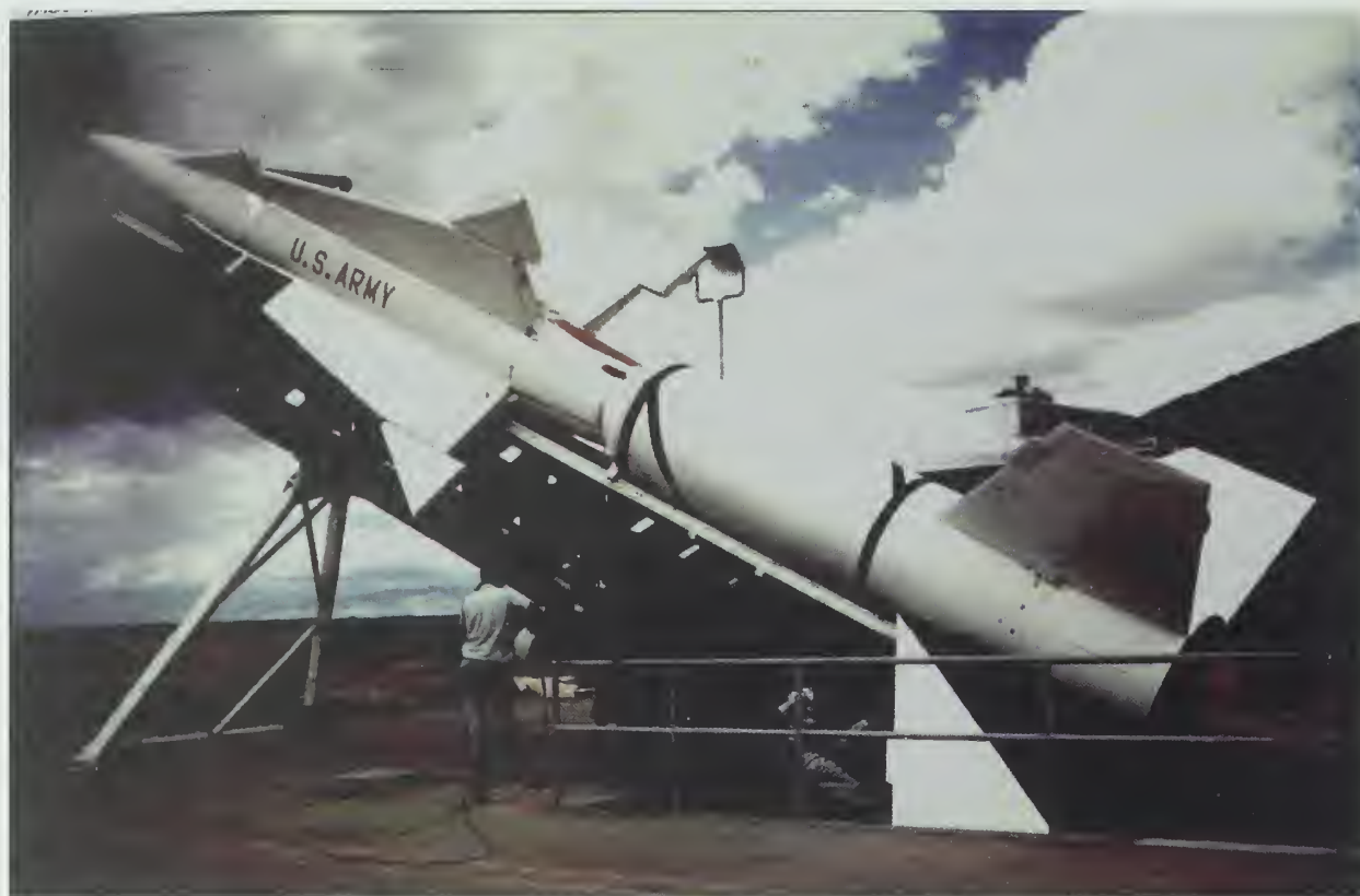
Fig. 2-10. A NIKE-ZEUS missile on a launcher during testing at White Sands Missile Range.
